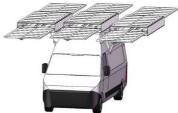
Fig 2 Photovoltaic panel deployment status
